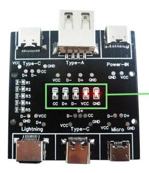
The VCC and GND indicators are on, indicating that the data line does not have the function of data transmission.
