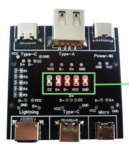
D+, D-, VCC, GND indicator lights are on, indicating that the data line has data transmission function.
