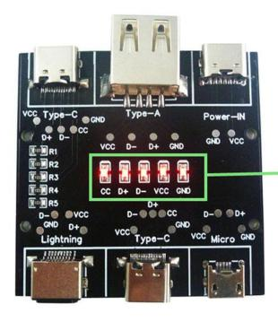
Type-c to Type-c data cable detection, CC, D+, D-, VCC, GND indicators are on. When testing other data cables, the CC indicator does not light up.
