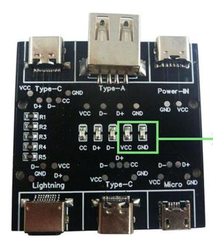
VCC or GND is off, indicating that the charging function of the data line is abnormal.
